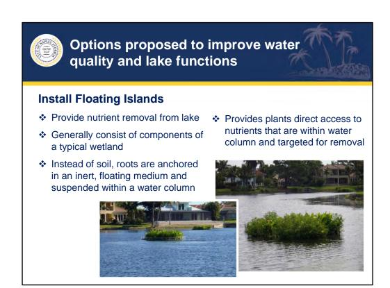
Floating islands provide nutrient removal from the lake and generally consist of components of a typical wetland. Instead of soil, roots are anchored in an inert, floating medium and suspended within a water column. This provides plants direct access to nutrients that are within the water column and targeted for removal.
