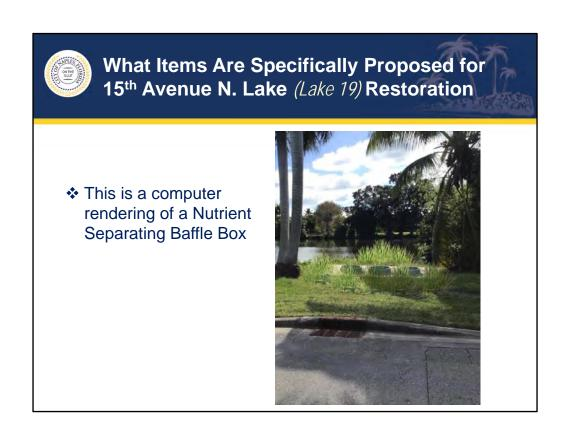
This is a computer rendering of a Nutrient Separating Baffle Box that will provide additional water quality improvements by capturing sediments prior to flows entering the lake.
