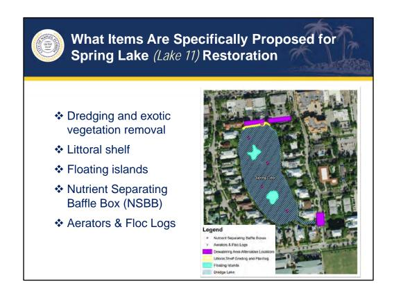
The specific improvements proposed at Spring Lake/Lake 11 include dredging, exotic vegetation removal, planting a littoral shelf, floating islands, a Nutrient Separating Baffle Box, and aerators with floc logs.
